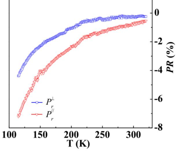
Here, PR is defined as PR=R<sub>light</sub>-R<sub>dark</sub> / R<sub>dark</sub>
