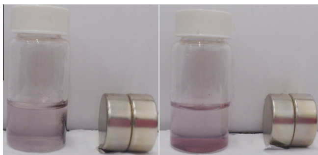
Fig. 7. Magnetic separability of as-prepared BiFe 0.95 Co 0.05 O 3 and BiFeO 3 . (The adsorbent can be effectively attracted by the magnet and accumulated in the left one.)
