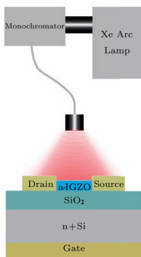
Fig. 1. Schematic of the device structure and the PECCS measurement setup.
