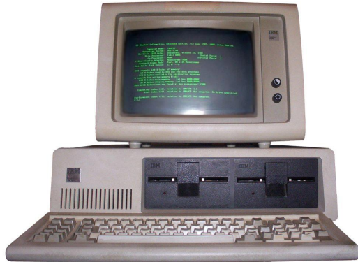
1981 IBM PC 5150 CPU: 8088, 5 MHz Floppy disk or cassette
